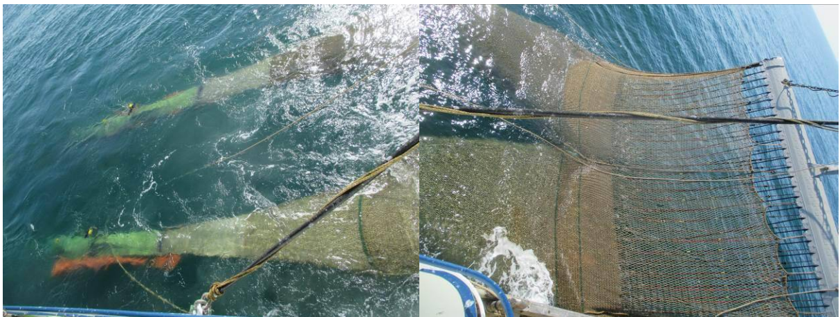
Figure 3. Left image shows the double cod-end of the port side trouser trawl with cod-end covers (green) and kites (black/yellow). Right image shows the Pulsing beam with electrodes.
