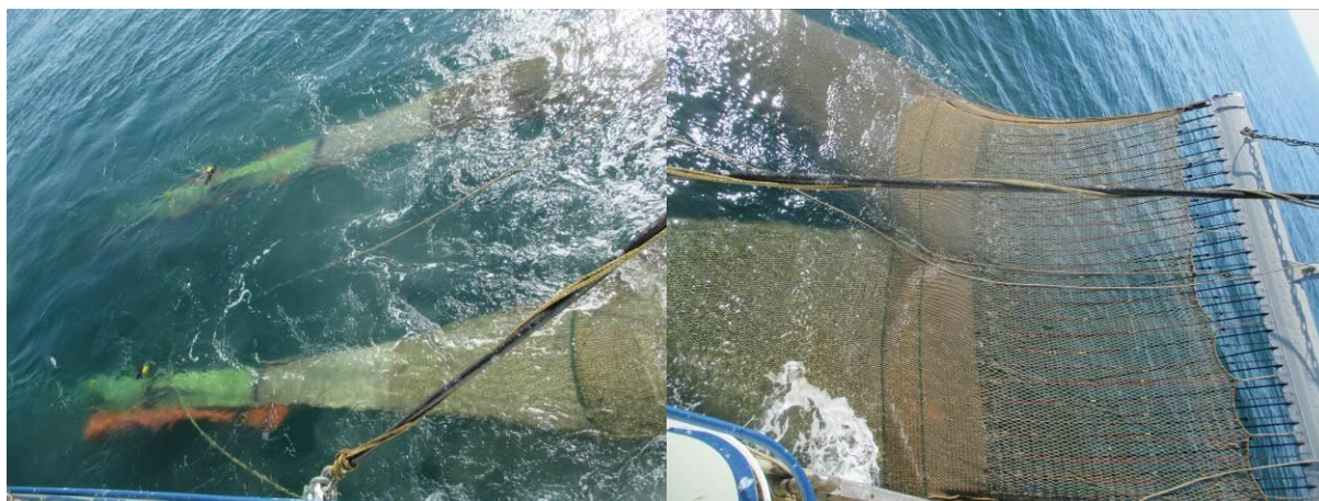
Figure 3. Left image shows the double cod-end of the port side trawl with cod-end covers (green) and kites (black/yellow). Right image shows the Pulsing beam with electrodes.
